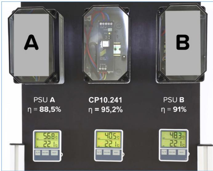
Figure 1: Experimental setup after a 4-hour runtime
